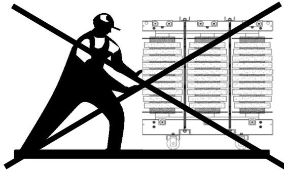
Move the transformer, whether alone or enclosed in an integral sheet metal box, by leverage against lower clamps or by means of its towing holes only.
